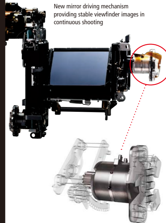
Mirror stepping motor's assistance The motor accelerates the initial mirror-up and -down movement, speeding up the whole process. It also decelerates the mirror-down movement just before it's completed, in order to minimize mirror bounce.
